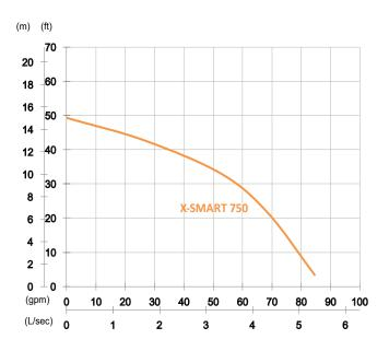
Shaft Speed: 3450 rpm Outlet: 50mm, 2in
