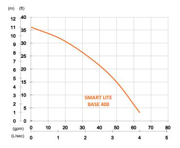
Shaft Speed: 3450 rpm Outlet: 50mm, 2in
