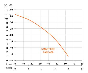
Shaft Speed: 2850 rpm Outlet: 50mm, 2in
