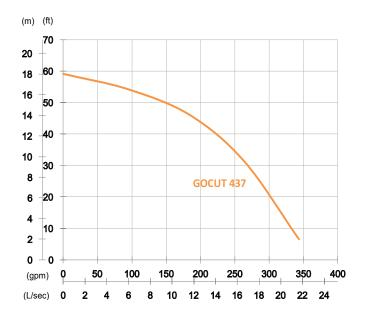
Shaft Speed: 2850 rpm Outlet: 100mm, 4in
