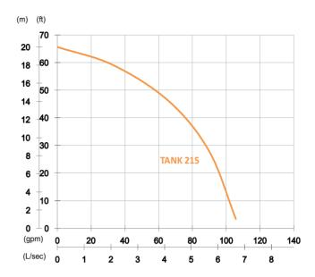
Shaft Speed: 2850 rpm Outlet: 50mm, 2in
