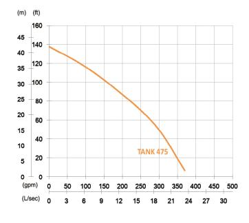
Shaft Speed : 2850 rpm
