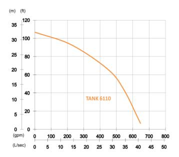
Shaft Speed: 2850 rpm Outlet: 150mm, 6in
