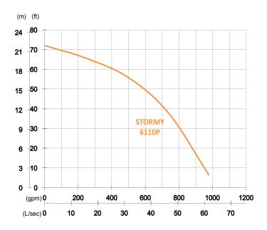
Shaft Speed: 1750 rpm Outlet: 150mm, 6in
