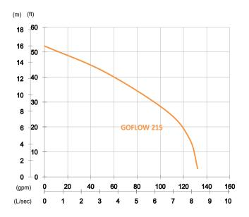
Shaft Speed: 2850 rpm Outlet: 50mm, 2in
